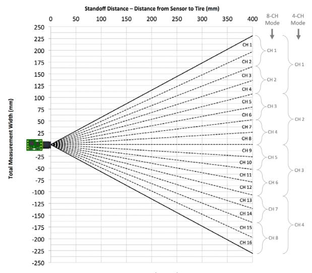
(Approximate. Angle offset (z-axis rotation) between -5° and +5°, mounts should allow adjustment accordingly)
