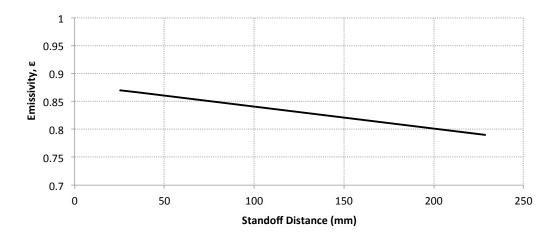
o Lowering the emissivity increases the measured object temperature and vice versa
