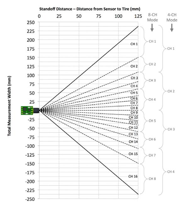
(Approximate. Angle offset (z-axis rotation) between -5° and +5°, mounts should allow adjustment accordingly)
